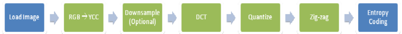
Figure 4: In the implementation of the baseline JPEG standard using color cameras, Bayer interpolation is first used to render the image in RGB space. Images are then transformed from RGB to YUV color space, DCT applied followed by quantization, zig-zag re-ordering and run-
